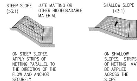
WHERE THERE IS A BERM AT THE TOP OF THE SLOPE, BRING THE NETTING OVER THE BERM AND ANCHOR IT BEHIND THE BERM
